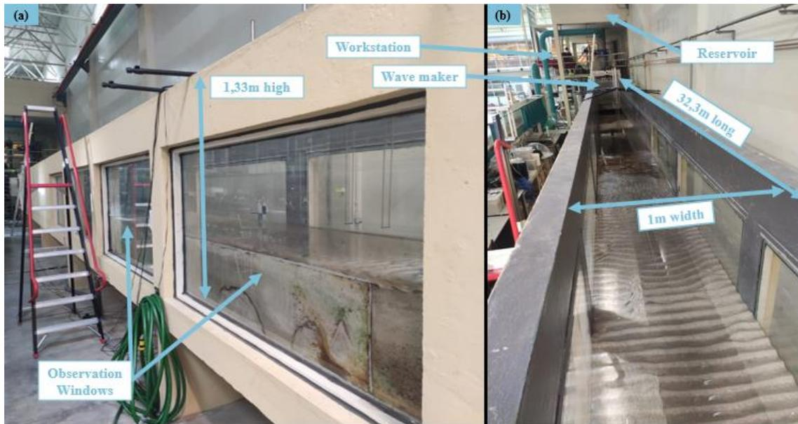
Figure 48. Dimensions of the channel used.
