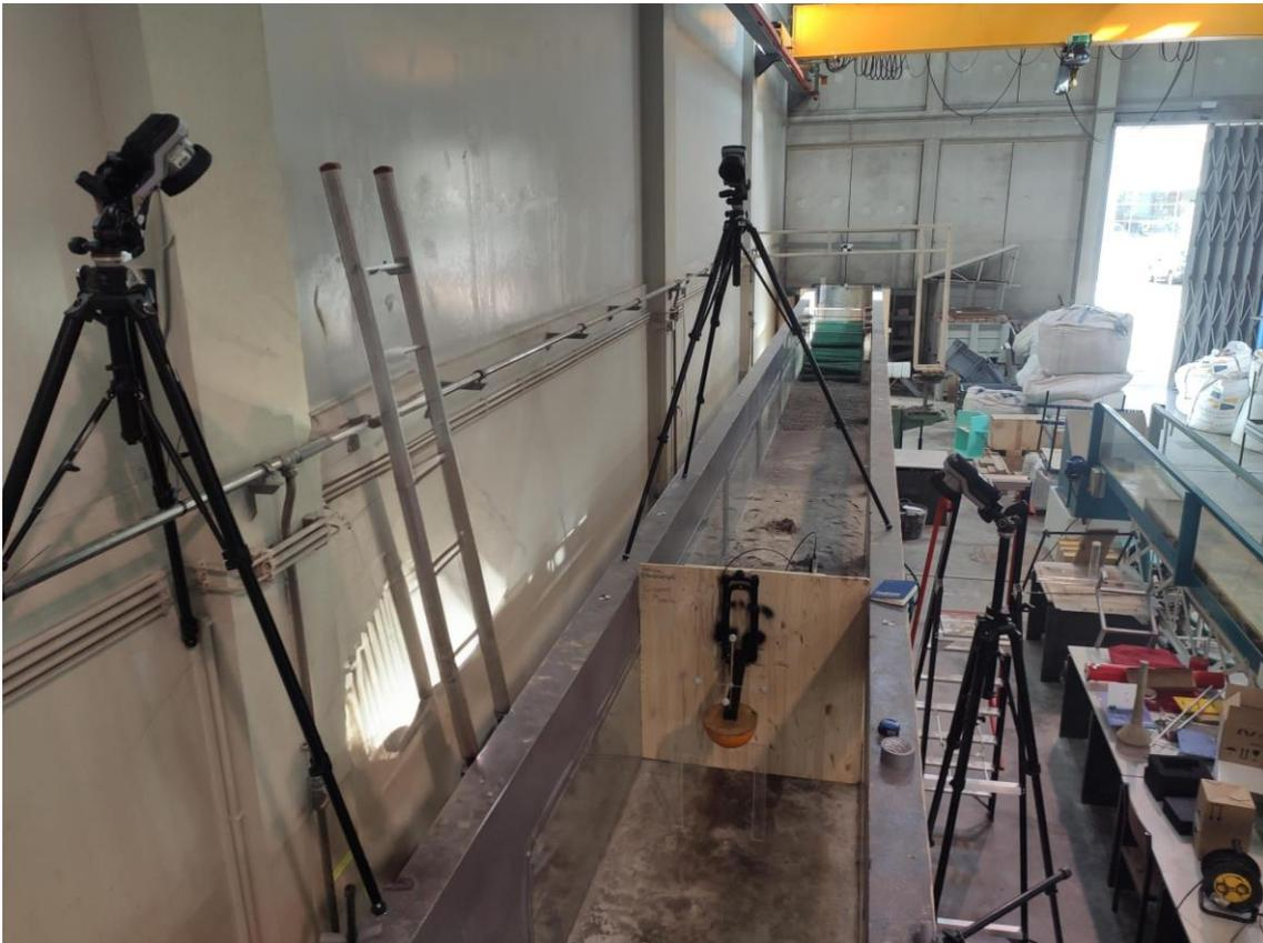
Figure 53. Qualisys® cameras setup and positioning.
