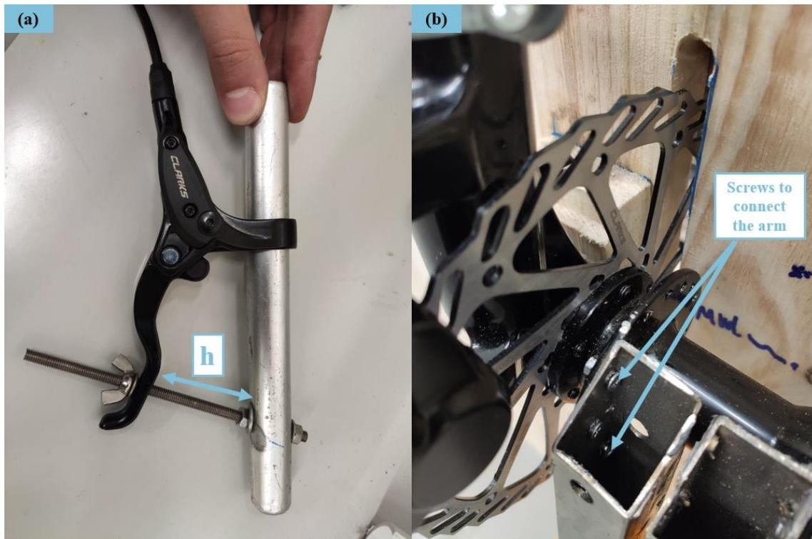
Figure 47. Detailed view of the arm attachment zone and brake setup.
