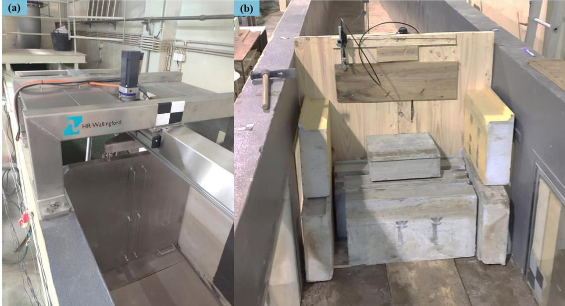
Figure 55. HR Wallingford® wave maker and concrete blocks used.
