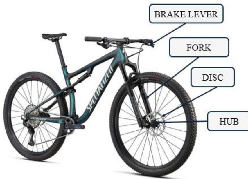
Figure 45. Bicycle components used for experimental modeling.
