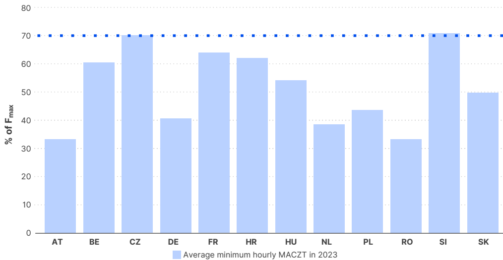
Figure 17: Average minimum hourly margin available for cross-zonal trade in the Core CCR for each Member State, considering flows induced by third-country exchanges – 2023 (% of F_{max} )
