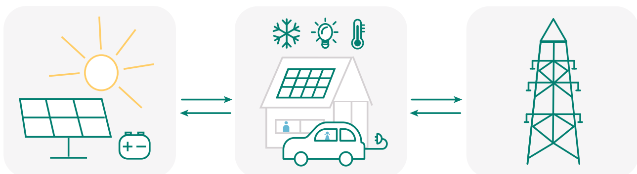
Figure 3.1 Schematic diagram of a possible prosumer household
