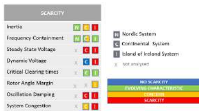
Figure 47 Technical scarcities’ forecast for 2030 in 3 European synchronous systems of the EU-SysFlex project 244
