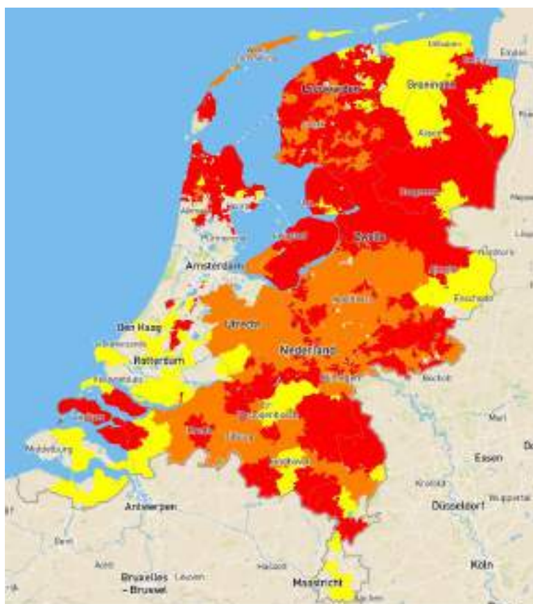
Figure 46 Capacity map of the Dutch electricity grid as of 14/04/2022 (injection) 221
