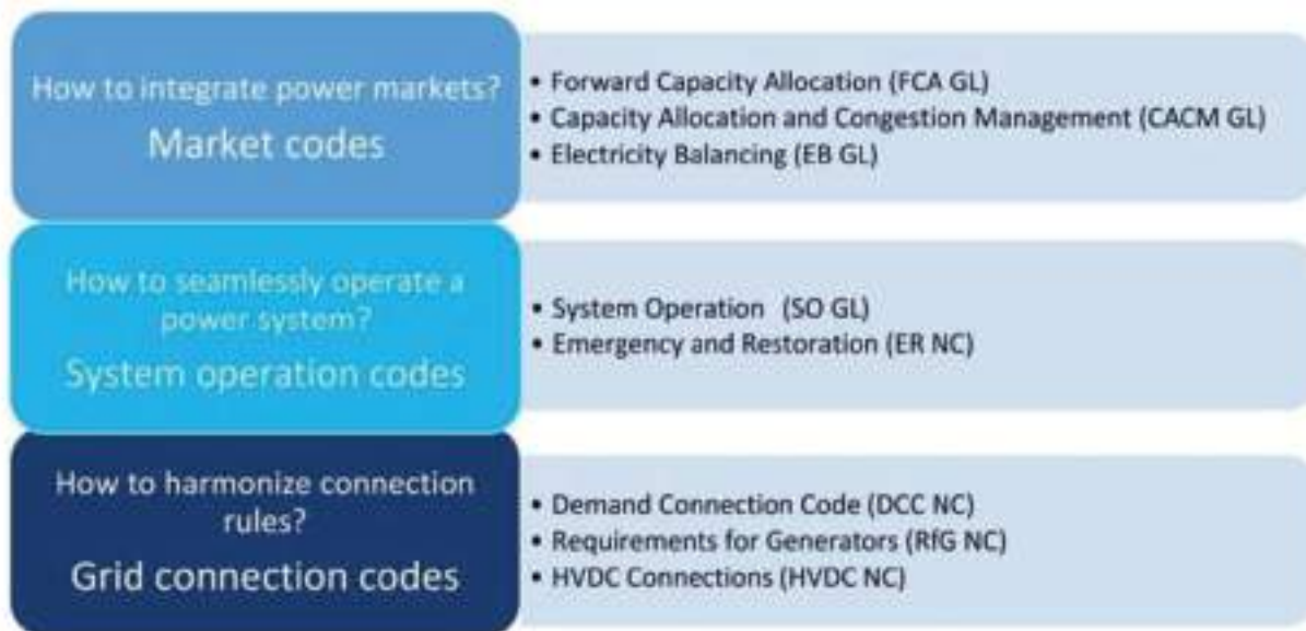
Figure 28: Electricity network codes and guidelines. Own illustration
