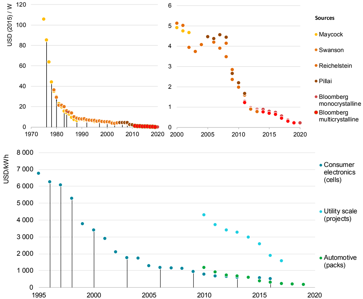
Figure 3.7 Evolution of solar PV module cost (top) and Li-ion battery price (bottom)
