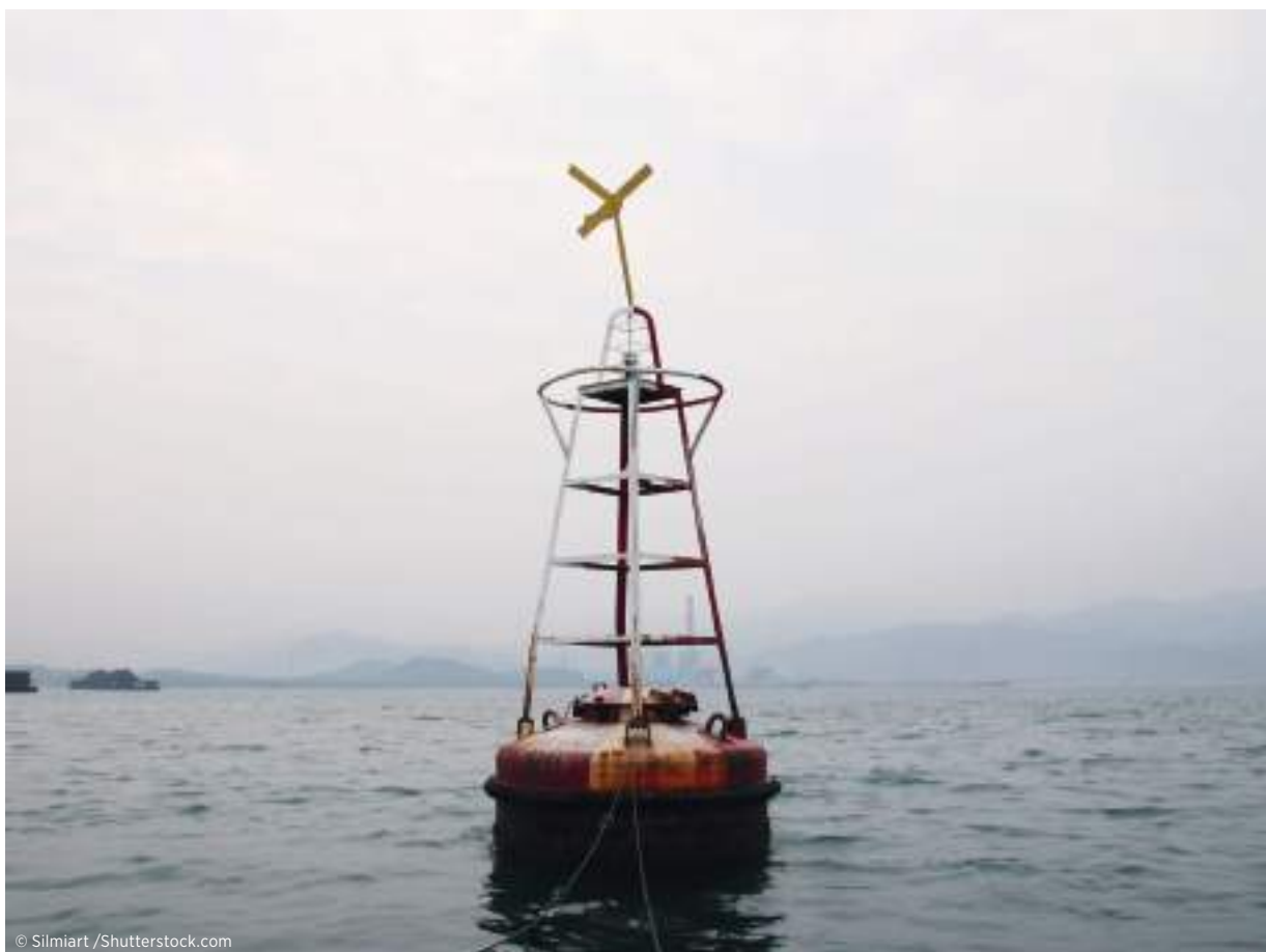
Wind- and solar-powered earthquake and tsunami observation system
