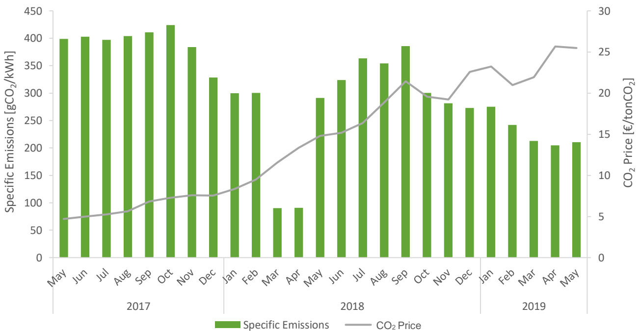
Figure 3. Specific emissions resultant from the power sector's activity in Mainland Portugal and CO 2 allowances price (May-2017 to May-2019).
