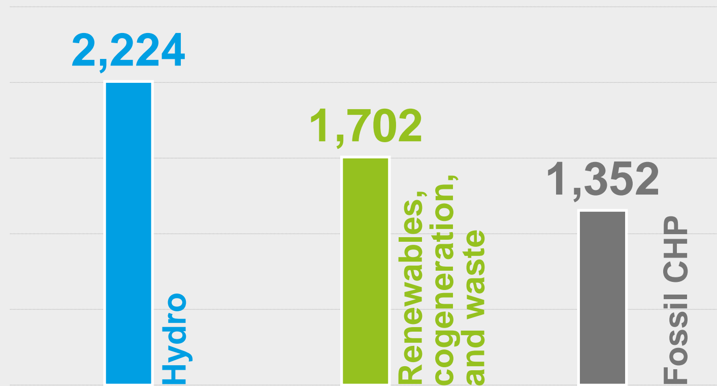
Number of market price setting hours of the three main market setting technologies (Jan-2023 to September-2023). Source: OMIE. Analysis APREN
